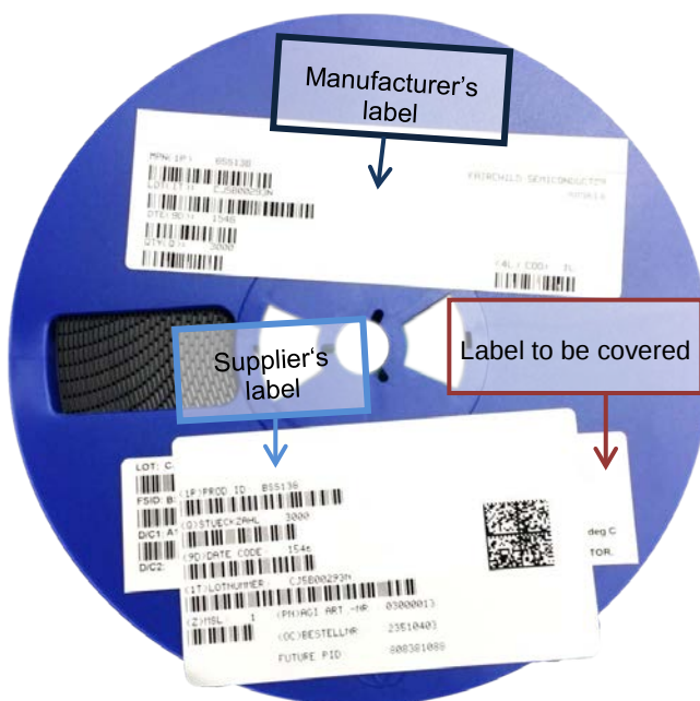
Picture 4: Correct covering shown on the example of a component roll
