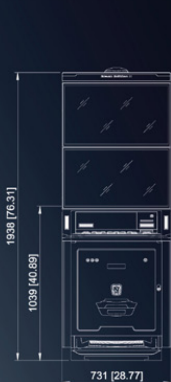
BLACK EDITION II XL 2.32/3.32 (FV837B) All dimensions in mm [in] · scale 1:25
