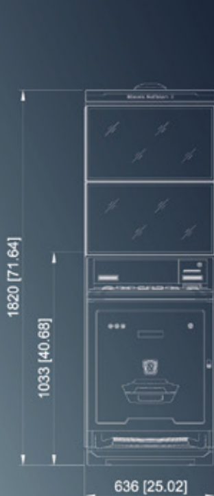
BLACK EDITION II 3.27 (FV837A) All dimensions in mm [in] · scale 1:25
